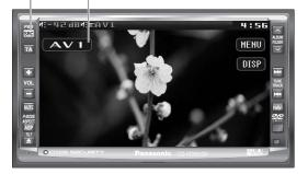
To switch Operation Screen ON, touch the center of touch panel or press [ENTER] on the remote control.
